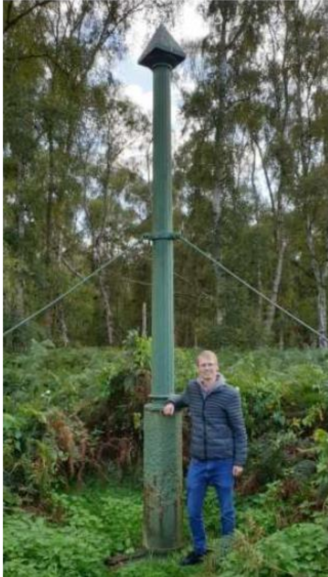
Figure 1: The Holme post at Holme Fen, Cambridgeshire. Driven into the peat in 1851, the posts' top marked the ground level, 4m higher than present day. (Photo - Page, S) (Page et al., 2020)
